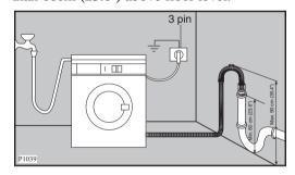
The drain hose may be extended to a maximum of 4 metres. An additional drain hose and joining piece is available from your local Service Force Centre. The joining piece must have an internal diameter of 18mm. If your drain hose looks like this (see below) you do not require the "U" piece". Just push the hose firmly into
